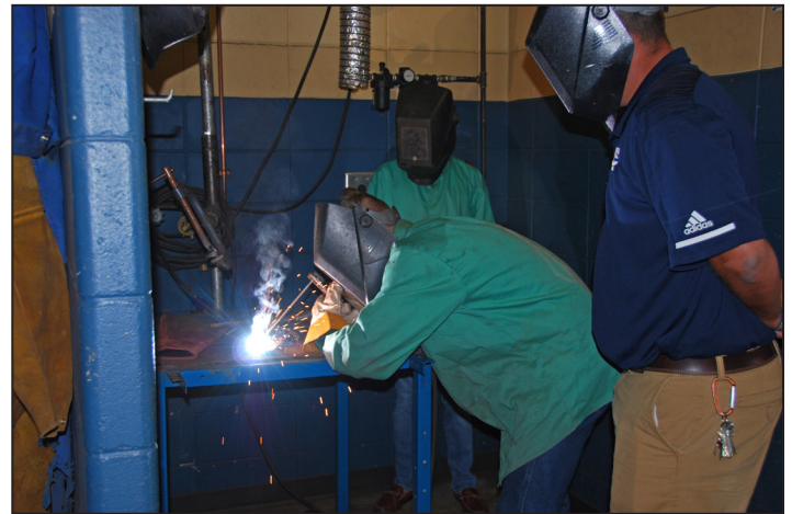
TCCHS students Douglas Hopkins, from left, and Lang Stringer use 6011 welding rods to learn stick welding techniques from welding teacher Travis Barrett.
